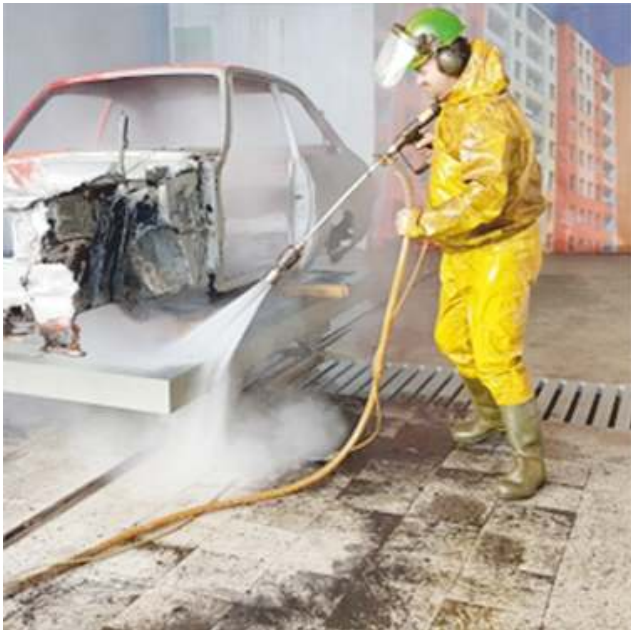
HIGH PRESSURE WATER JET CLEANING
